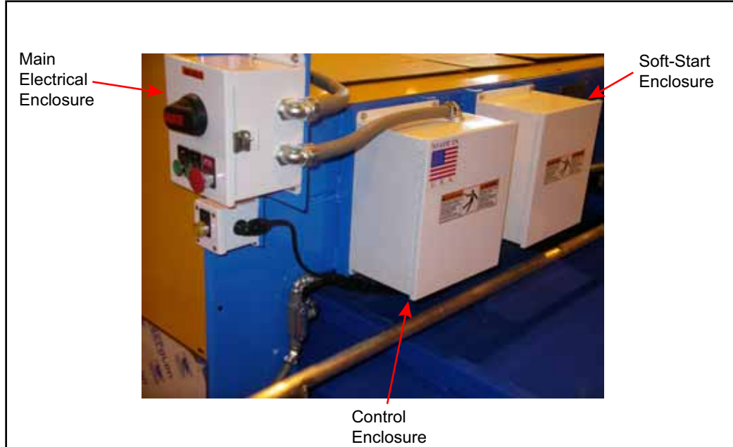
Figure 4: Soft-Start and Control Enclosures
